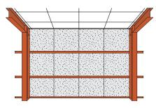
Cut unfaced, uncompressed insulation to fit the exact height between girts, plus one inch extra. Impale insulation onto Fast-R hangers throughout the wall area, filling the girt cavities.
