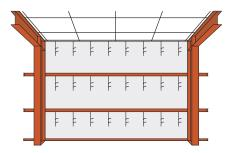
Apply Quik-Stop thermal break tape to exterior girt flanges prior to installing exterior metal wall panels. From the interior of the building, install Fast-R rigid insulation hangers as specified.
