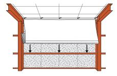
Position appropriate sized Syseal air barrier fabric in wall area. Fabric positioned from ceiling to floor and from column to column.
